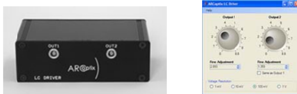
USB LC driver with two independent outputs and software
