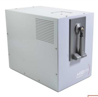
The ARCoptix VIS-NIR-DR spectrometer is a broadband instrument designed for diffuse reflectance measurements in the visible and near-infrared. The entrance port of the instrument leads to an integrating sphere with internal illumination, which ensures optimized illumination of your sample. The VIS-NIR-DR integrates a multichannel grating spectrometer for measuring in the visible as well as an FT-IR that covers the NIR region of the electromagnetic spectrum.
