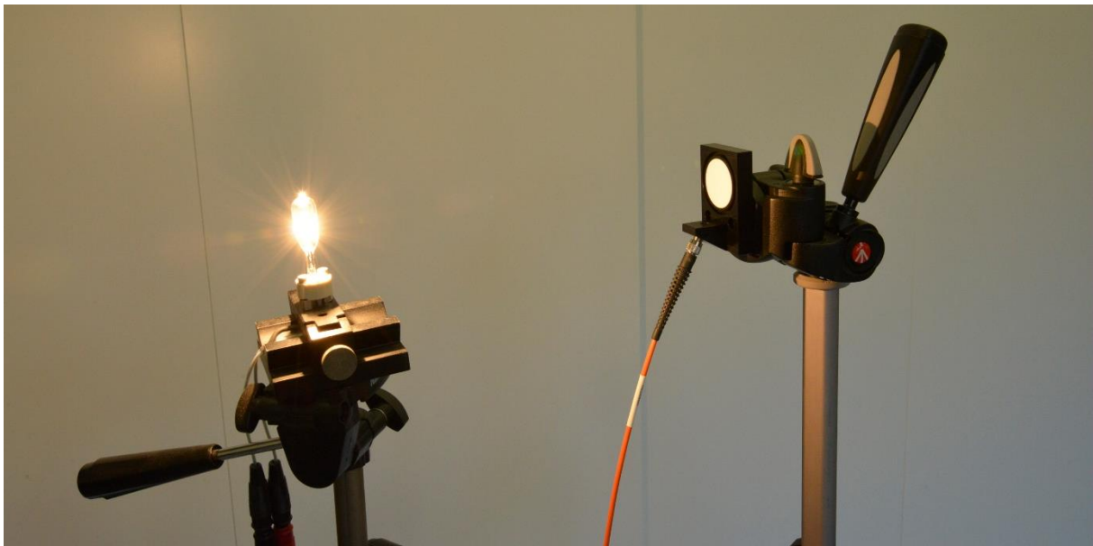
Figure 2 - Irradiance calibration set-up, including the Arcoptix Reflective Cosine Receiver
