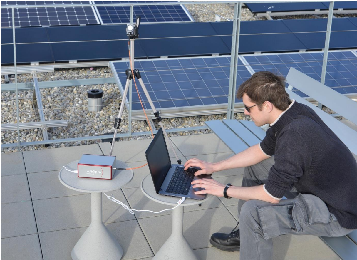
Figure 4 - Outdoor solar irradiance measurement. The spectrometer, reflective cosine receiver on a photographic tripod, and laptop computer.
