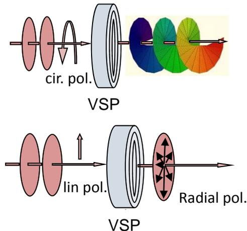
By introducing an additional variable phase retarder in front of the VSP all kinds of polarization distributions and phase plates can be generated. When adjusted at quarter wavelength it transforms the linear polarization in circular one and the VSP plate will transform this planar beam into a spiral phase beam.
