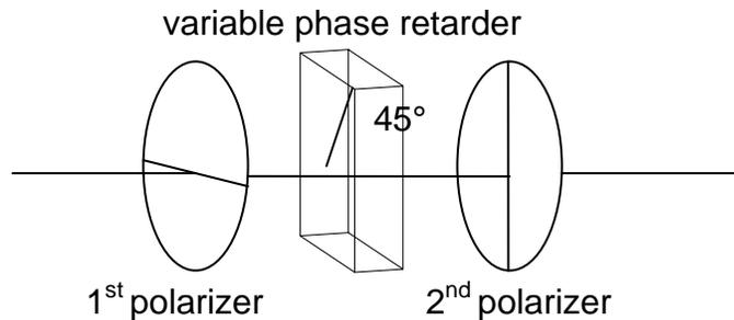
*Variable attenuator composed of a variable phase retarder between crossed polarizers.*
